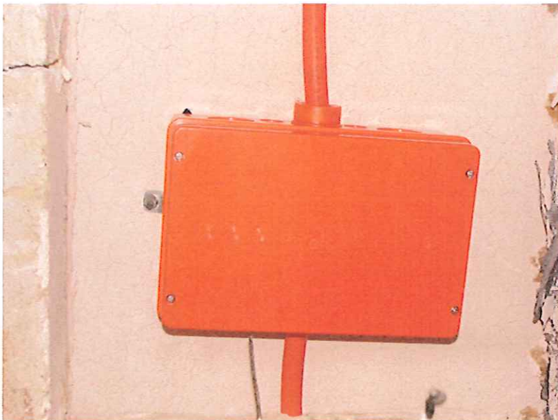
Photo 2: test sample "WKE 5" (closed) before fire test according to DIN EN 12101-3: 2002
